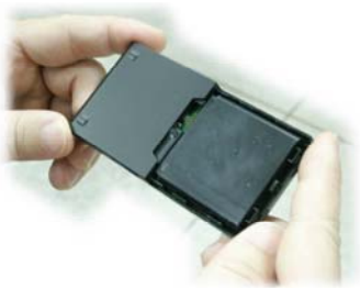
Step 2 Open the cover of battery
