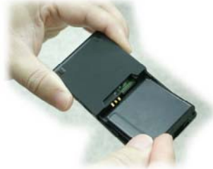
Step 4 Fit new battery into iBT-GPS
